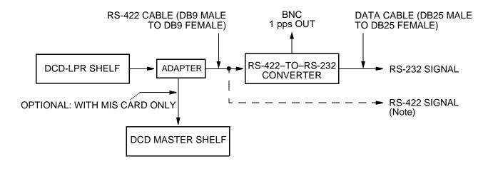
Note: RS-422-to-RS-232 converter not required for RS-422 signal.
